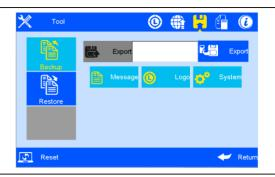
Clip Restore to enter the backup restore interface; can restore the message, image and setting of USB disk to the device;
