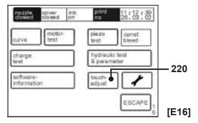
The display is adjusted with the **<adjust>** field (221) and by tapping on the upper calibration point (222) and by subsequent tapping on the lower calibration point (222). The storage is performed with the touch field **<save>** (223).
